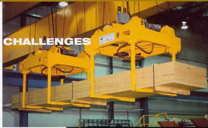
This lumber grapple was designed for both single-sheet and multi-sheet handling.
