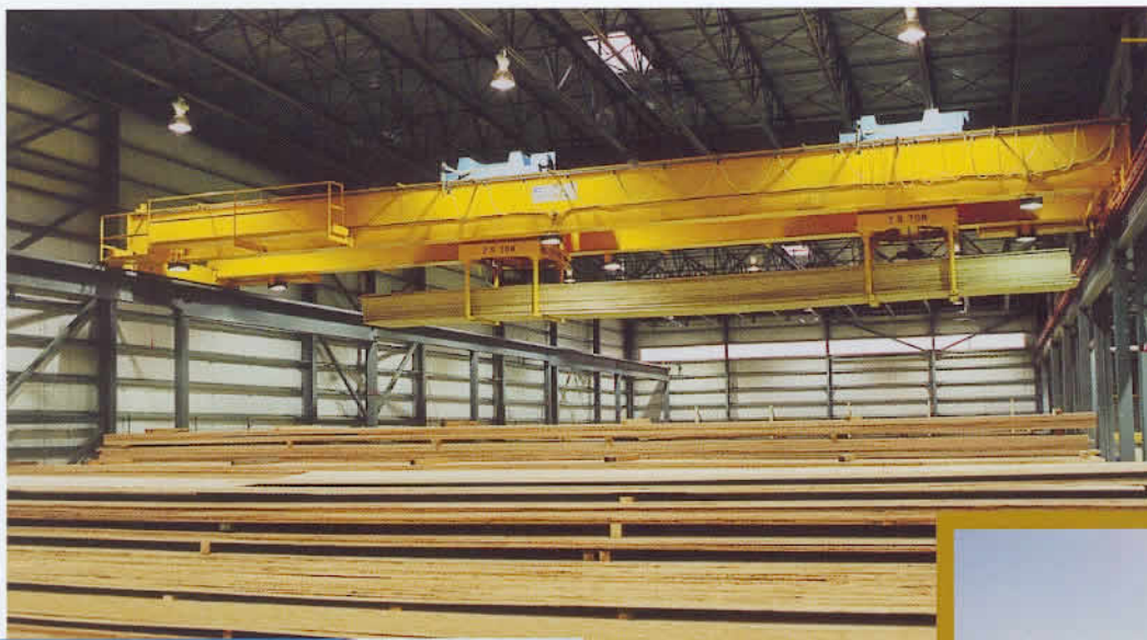
This overhead crane was custom built for an LVL manufacturer in the U.S. The wood sheets measure 60 feet long and four feet wide.
