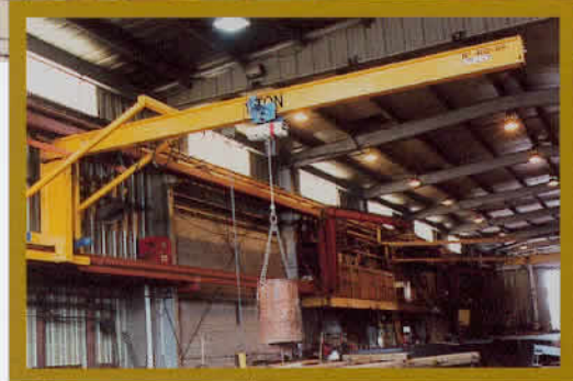
Low head room wall running jib crane.
