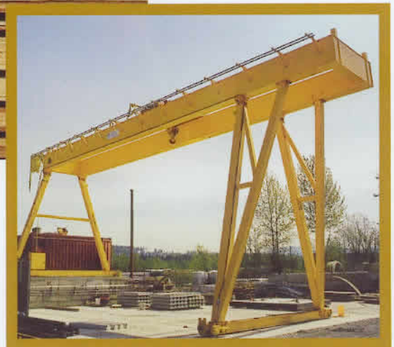
A unique feature on this double-girder gantry crane is the uneven legs. The client preferred to have one leg sit on an elevated block to prevent some mechanical equipment from getting clogged by dirt.
