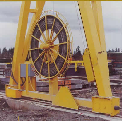
This cable reel, driven by a counterweight, operates on relatively low-tech engineering principals. The simplicity of design ensures virtually trouble-free operation.
